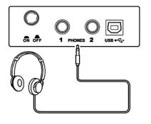
To the left beneath the keyboard you find the headphones outlets 1 and 2. Connecting headphones (not supplied) to outlet 2 mutes the speakers. Using outlet 1 maintains the sound output through the speakers.
