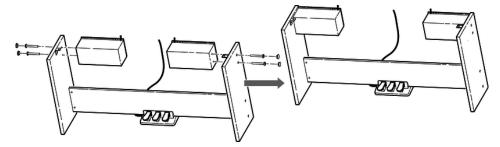
Attach the speakers with each two screws  $6\times 50$  to the side panels and cover the screws with screw caps.
