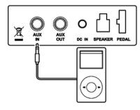
Use the AUX IN socket to connect a, for example, CD or MP3 player to the digital piano. So you can playback music through the internal speakers of the digital piano and simultaneously play along to it. Plug one end of the audio cable into the AUX IN socket on the rear panel of the digital piano and the other end into the output of the respective audio device.
