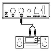
Use the AUX OUT socket to connect the digital piano to an amplifier, stereo device, mixing console or recording device. Plug one end of the audio cable into the AUX OUT socket on the rear panel of the digital piano and the other end into the input of the respective audio device.
