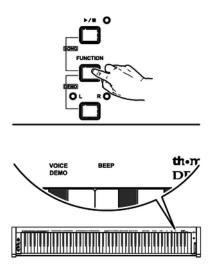
With this function, you can turn the Key Tone on or off. By default, the Key Tone is turned on. Keep the *[FUNCTION]* button pressed and press the piano key *[BEEP]* to turn the Key Tone on or off.
