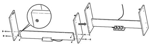
Insert the four Phillips-head barrel nuts (12) into the rear panel of the pedal box as shown in the left part of the figure. Use two screws  $6 \times 50$  on each side to attach the two side panels to the pedal box and cover the four screws with screw caps.
