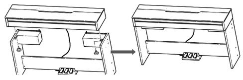
Put the digital piano housing on the stand and affix it using the two hand screws.
