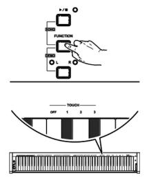
With this function you can adjust the touch response of the keyboard at four different levels.
