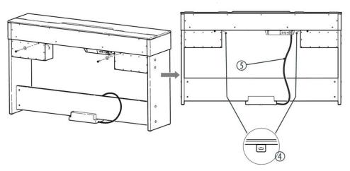
First fix the two speaker boxes with one screw each  $4\times15$  and the associated seal on the digital piano housing.
