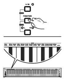
You can call up to 26 voices via the piano keys in the [VOICE] area. Each piano key in the [VOICE] area is assigned to two voices. With the first keystroke you activate the voice that is given in the first row above the button, with the second keystroke you activate the voice that is specified in the second line above the key.
