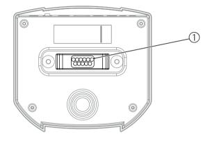
Multiple socket for connecting the pads
