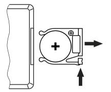
Push the lock of the battery holder towards the centre of the housing and pull out the battery holder like a drawer. Insert the batteries. The battery is correct if the positive pole points to the housing base of the remote control. Slide the battery holder back into the remote until it clicks into place.
