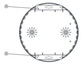
A Mounting tabs for ceiling or wall mounting of the unit.
