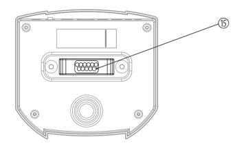
15 Multiple socket for connecting the pads.
