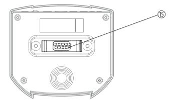
Multiple socket for connecting the pads.
