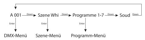
Press [DOWN] while 'A001' is flashing in the display to call up the preprogrammed scene. Press repeatedly [DOWN] to call one of the 7 programmes. If necessary, press repeatedly [DOWN] to set the device to sound-to-light mode.
