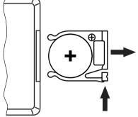
When shipping, the battery is already installed in the remote and protected against discharg by a transparent plastic foil. Remove the plastic foil prior to first use.
