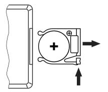
Push the lock of the battery holder towards the centre of the housing and pull out the battery holder like a drawer. Insert the batteries. The battery is correct if the positive pole points to the housing base of the remote control. Slide the battery holder back into the remote until it clicks into place.
