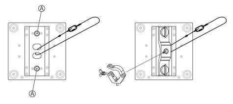
The threads on the bottom side of the housing (A) allow the secure attachment of the included mounting bracket. There, you can fasten adapters such as half couplers, trigger clamps, c-hooks etc. The safety cable is threaded through the cut-outs on the bottom of the housing.
