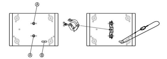
The threads on the bottom side of the housing (A) allow the secure attachment of the included mounting bracket. There, you can fasten adapters such as half couplers, trigger clamps, chooks etc. Safety cables are being threaded through the eyelet (B) on the bottom side of the housing.
