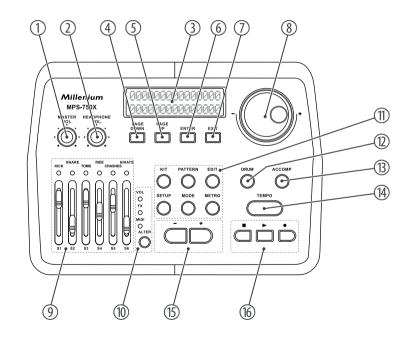
MPS-750X E-Drum Module
