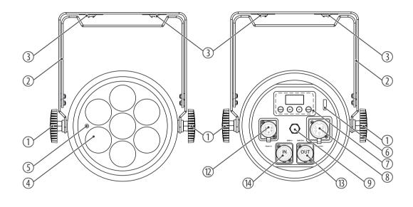
1 Locking screws for the brackets. 2 Two-piece bracket for hanging or floor setup 3 Omega bracket with quick lock fastener 4 LED 5 Infrared sensor for optional remote control 6 Safety cable eyelet 7 Display and keypad [MODE] Activates the main menu, toggles between the menu levels or closes a submenu. [DOWN] Decreases the displayed value by one. [UP] Increases the displayed value by one.
