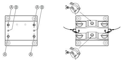
The Quick Lock mounts on the bottom side of the housing (A) allow the secure attachment of the included mounting brackets. There, you can fasten adapters such as half couplers, trigger clamps, c-hooks etc. Safety cables are being threaded through the safety eyelets (B) on the bottom side of the housing.
