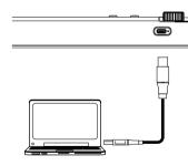
You can use the USB interface to connect the device to a PC via the supplied USB cable. As well as data transmission, this interface provides the power supply to the device and charges the built-in battery.
