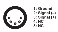
DMX-input XLR mounting-plug:
