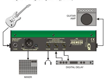
The SEND & RETURN are being used to divert the sound through an external delay processor. The delay is then switched off when the gbQ's 'BYPASS' footswitch is pressed. The DI Output provides a separate feed to the PA System.
