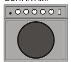
INPUT – sets the gain of the preamplifier, to match the guitar to the guitar amplifier.
