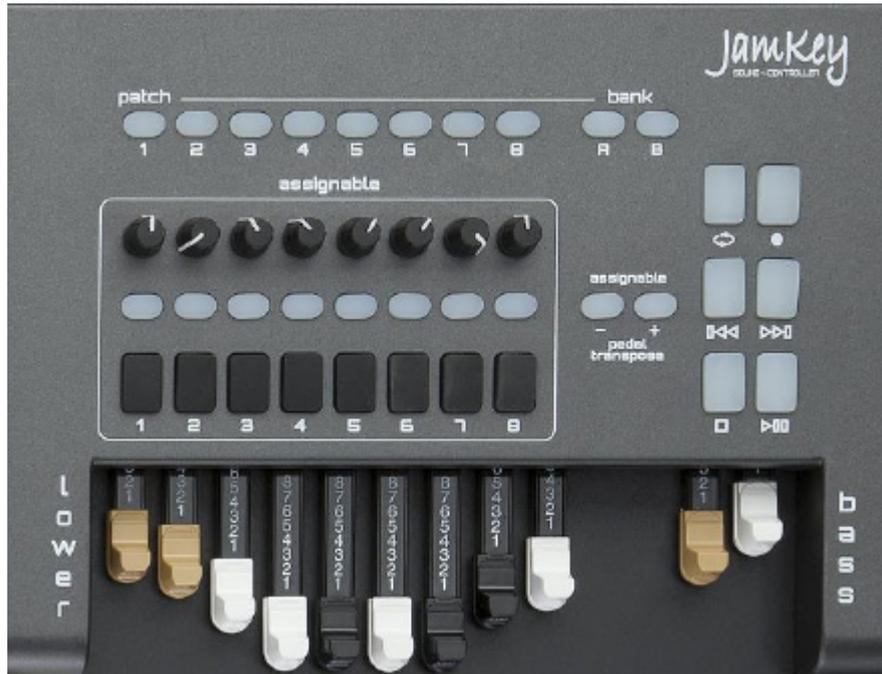
On the Right control panel there are 8 rotary knobs. They can be programmed for different functions.
