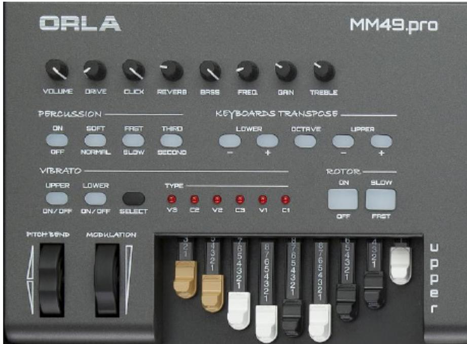
On the left control panel there are 8 rotary knobs. They are assigned by default to the Drawbar Organ features but can be reprogrammed for new functions.
