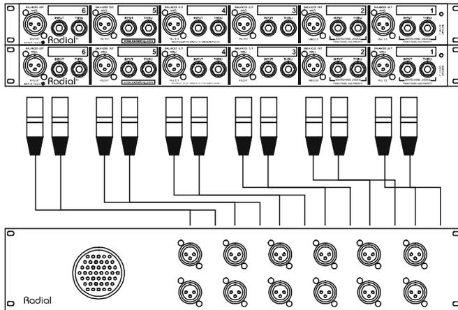
The second JD6-X12 panel is designed for use when using 12 channels or two JD6's together in a rack. A 37-pin multi connector is used in conjunction with a multi-pin to XLR male breakout or multi-to-multi. This handy quick-disconnect option accelerates system set-ups and tear-downs by allowing 12 keyboards connections to be made with a simple 1/4" twist!
