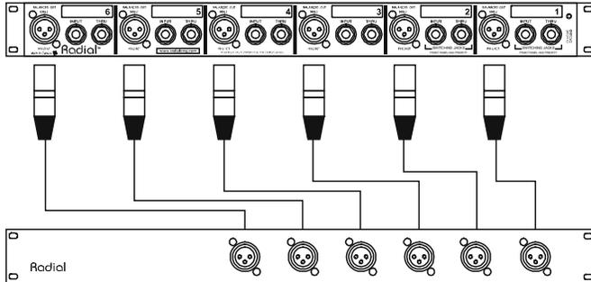
This top figure shows the JD6 with a simple XLR breakout panel called the JD6-X6. This comes standard with 3 feet and 6 feet extensions allowing the breakout panel to be mounted on the back or the front of the keyboard rack.
