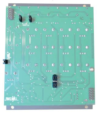
Single Pressure Points with no BRAINS attached. Note all the "Close 4 Master" locations are closed, as well as the Expand headers.
