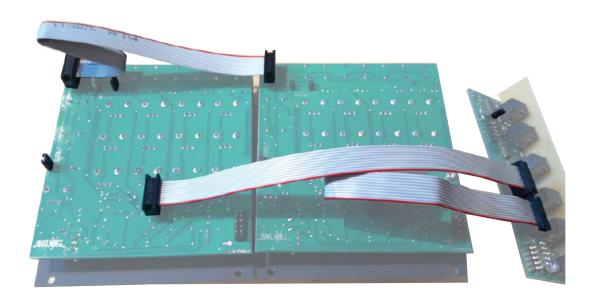
**BRAINS** with two Pressure Points:Two is the maximum number of Pressure Points that can be attached to a single **BRAINS**. Note: the connections of "Points 1-4" and "Points 5-8" to EXPAND headers the single open location on the "Master" Pressure Points' "Close 4 Master" headers; all three "Close 4 Master" locations open on the non-master Pressure Points, and the Jumper on BRAINS set to "2PP."
