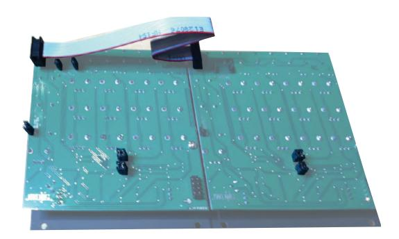
Two Pressure Points, chained. Note that the "Close 4 Master" headers are closed on the first unit (will be on the right when installed in the case). For three or four Pressure Points, use 4-header CHAIN cable and leave "Close 4 Master" headers open on all units but the master (rightmost when installed/leftmost from behind). Also, note the jumpers on the EXPAND headers.
