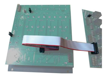
**BRAINS with a single Pressure Points:** Note the single open "Close 4 Master" header, the BRAINS cable connected from "Points 1-4" header to EXPAND header, and the jumper on BRAINS set to "1PP."
