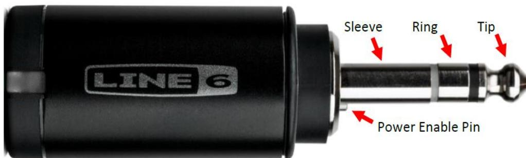
A typical guitar output jack, shown at right, has a threaded sleeve, a contact point to electrically connect to the tip of the plug, and an electrical connection to the sleeve of the plug. When the G10T is inserted, the power enable pin will be pushed in by the jack's sleeve edge, which will turn on the power of the G10T.
