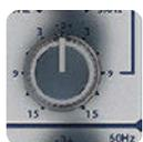
This will adjust the gain or attenuation of the audio band centred according to the MF Frequency. This is an asymmetric EQ, so boost has a wide bandwidth (low Q), and cut has a narrow bandwidth (High Q). See section 1.0.2 for more detail.
