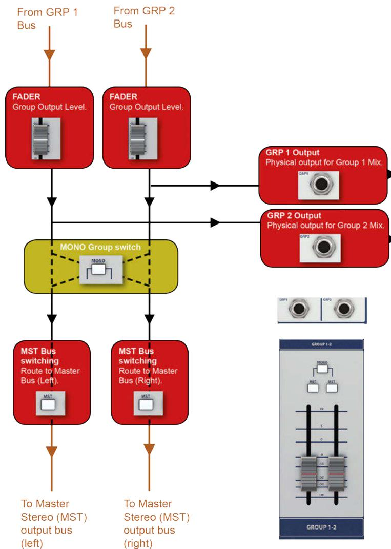
CONSOLE ROUTING > MASTER STEREO OUTPUT
