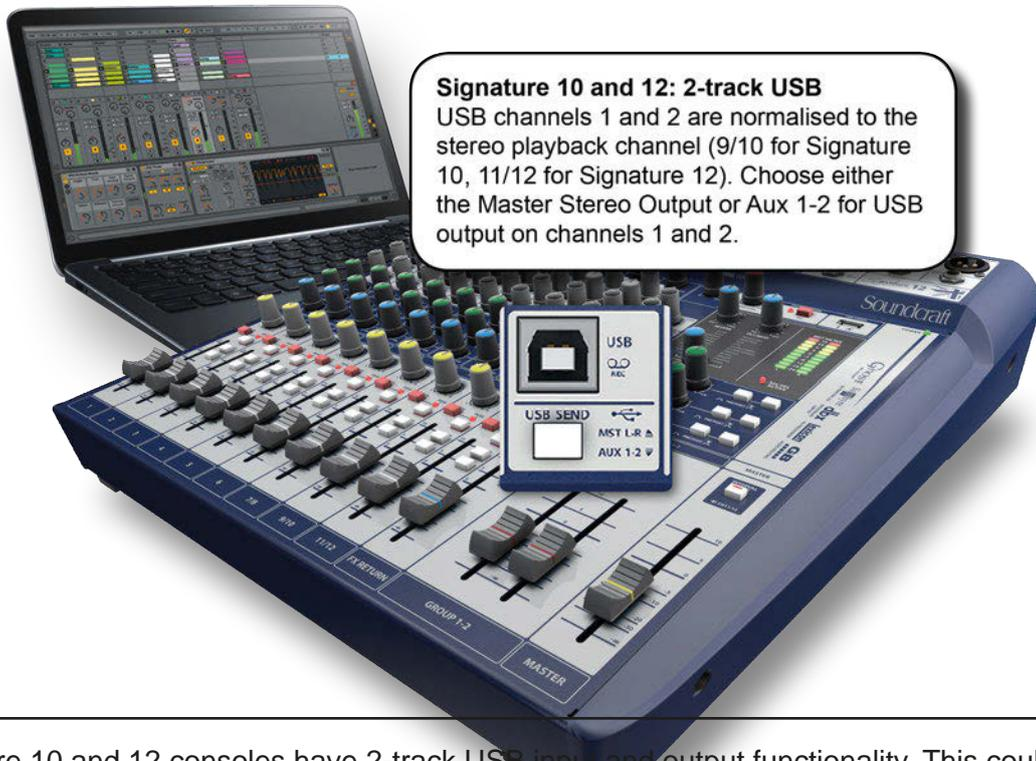
The Signature 10 and 12 consoles have 2-track USB input and output functionality. This could be used for recording a mix to a PC or Tablet, for example - or to use a computer as a playback device. Channels 1 and 2 are received by the highest-numbered stereo channel (9/10 for Signature 10, 11/12 for Signature 12).
