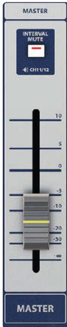
The Master (MST) Stereo Output channel determines the output level of the main stereo (left and right) mix from the MST L and MST R physical outputs.
