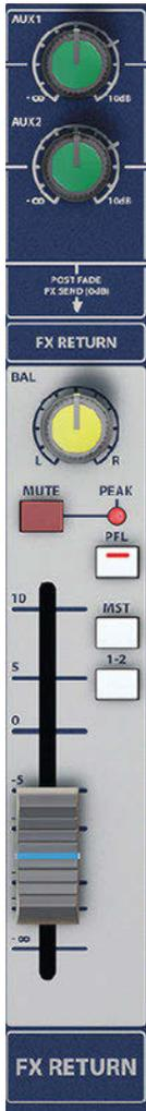
The stereo FX Return channel is fed from the output of the console's internal FX processor. It is a cut-down version of the normal stereo channel, without trim, EQ, or Aux 3 send.
