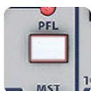
With a PFL enabled, the headphone output will switch to the Solo Bus. Please see section 6 for more detail.
