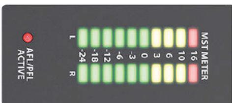
The meters on the Signature 10, 12, and 12MTK show Master Left/Right output level in normal operation. Refer to section 6.0 for more detail. The AFL/PFL ACTIVE indicator is below the main meters and lights when any AFI or PFL selection is engaged. See section 6.0 for more detail.
