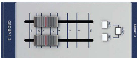
The Group Output Master channels control routing and output level for the Group busses. For Signature 12 and 12MTK Group 1 and 2 outputs can be summed to mono and/or routed to the Master Stereo Output. Refer to Sections 4.6 and 5.6 for more detail.
