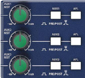
Aux (Auxiliary) Master output channels control the output level of the auxiliary bus and global pre-fade/post-fader switching. AFL switching allows aux master solos. Refer to Sections 4.5 and 5.5 for more detail.
