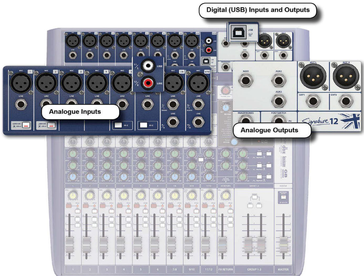
INPUTS & OUTPUTS > INTRODUCTION TO I/O
