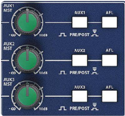
The Aux Master Output channel determines the output level of a whole Aux mix (the sum of all Aux contributions). That is, the Aux 1 Master controls the Aux 1 output level, which is the sum of all Aux 1 contributions from the input channels.
