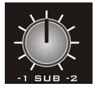
Left; changes the level of VCO1 Sub, which is one octave down from VCO1.
