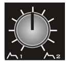
This control routes either envelope to modulate the frequency cutoff. The centre position is off/no modulation. Modulation can be either EG1 (left) or EG2 (right).
