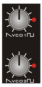
Left; changes the level of VCO1 Sawtooth waveform. RIght; changes the level of VCO1 Square waveform.
