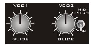
This is a portamento function. Each note will glide to the next new note, slowly rising or failing in pitch to the new note. The Glide knob changes the rate (time) it takes to reach the new note.
