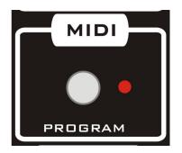
This button is used to set the MIDI channel and CV2 controller.
