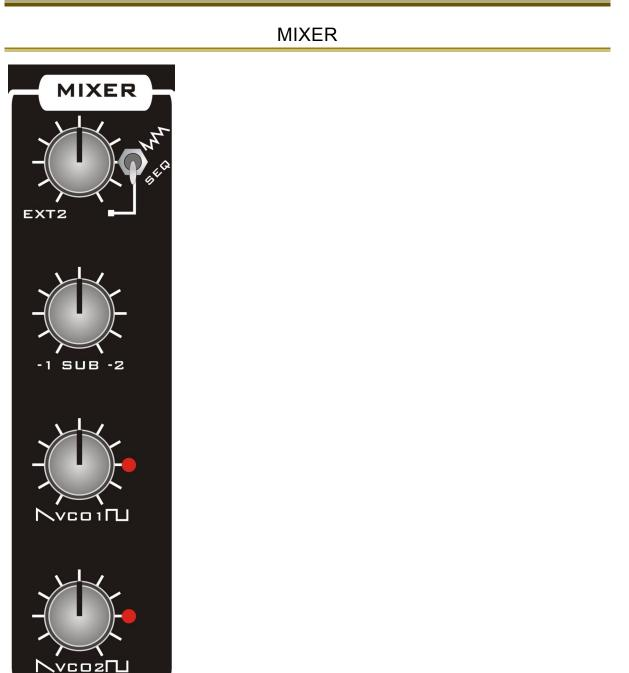
There audio is mixed with the mixer before being fed to the input of the filter.
