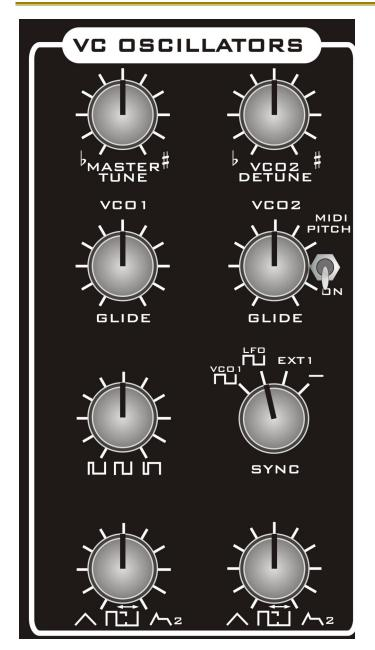
The two VCOs are almost identical, but VCO1 has a manual pulse width control, and VCO2 has a Sync feature.
