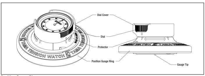
**Position Gauge Ring:** The Tension Watch comes with a Position Gauge Ring which enables you to keep a fixed distance from the hoop/tension rod to allow you to tune the drum with more consistency and accuracy.
