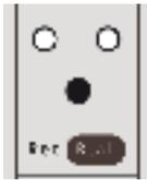
To enable Play mode, please hit the **Rec/Real** key. Both LEDs above should be idle now.
