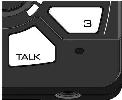
*The built-in microphone – right below the Preset 3 button*
