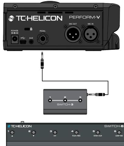
*Connecting a Switch-3 or Switch-6 to your Perform-V's pedal input*
