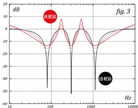
as six phase shifting stages. These outputs result in a 2-notch and 3-notch frequency response, respectively, and can be used as a faux stereo pair to widen and spatially animate the signal. Of course, the outputs can also be used independently, as they each have a unique character.
