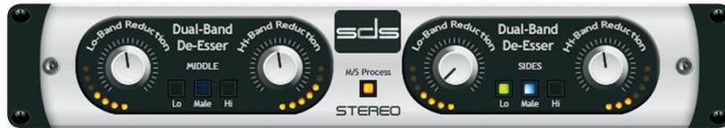
The **DE-ESSER** is a “must-have” tool for reducing the amount of sibilance in vocal mics while adeptly preserving the natural voice timbre of a performance. Use it to enhance the smoothness of the upper mid to high frequencies in vocals as well as drum overheads and strings, etc. (Inspired by SPL 1219\*)
