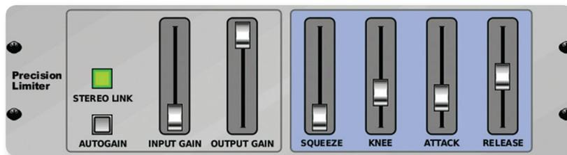
The **STEREO PRECISION LIMITER** is perfect for setting a precise volume limits, ensuring distortion-free and optimal signal integrity. Use the Stereo Precision Limiter to boost quiet signals or reduce the level of “hot” signals to prevent clipping. (Inspired by Sony Oxford Dynamics\*)
