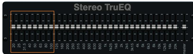
Unlike typical graphic EQs, our **STEREO TruEQ** delivers the exact frequency response for the new fader setting, taking neighboring fader settings into account – for surgical and responsive filtering or general room equalization (Modeled after BEHRINGER UltraCurve DEQ2496). The XR18 can provide up to 16 mono graphic EQs – one in each of the 6 Aux Buses and Main LR, plus 8 additional mono GEQ effects (4 stereo) that may be inserted into channels.
