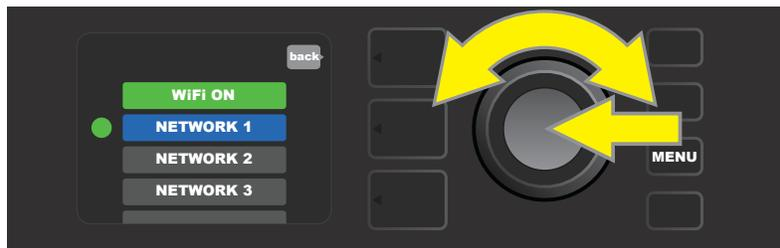
Once a network is chosen, select "CONNECT" from the menu shown by pressing the ENCODER on it:
