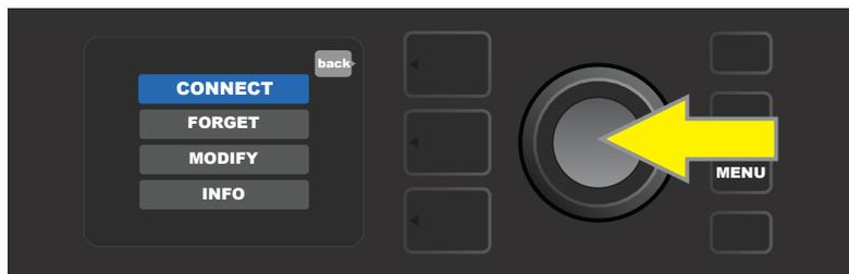
After choosing "CONNECT," the amp will then prompt entry of a password (*not shown*). To spell out a password, press the ENCODER once to activate the cursor and turn it to choose a character. Press ENCODER again to enter that character and move to the next; repeat until password is complete. When password is complete, press SAVE. Successful network connection is indicated by a green dot to the left of the network name.
