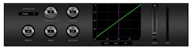
The **Compressor** comes with the standard Threshold, Ratio, Attack and Release knobs and allows Knee control. The Detector drop-down menu offers several Peak / RMS sense modes to choose from.
