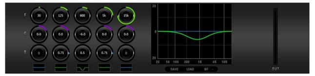
Antelope Audio's integrated **EQ** offers 5 fully parametric bands, two of those can work in filter or shelving mode and the three in the middle can cut or boost selected frequency ranges.
