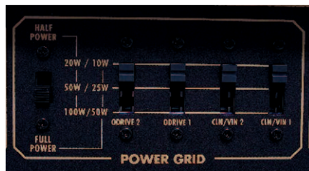
The Power Grid function allows you to select the wattage for each of the Tourmaster's four channels.
