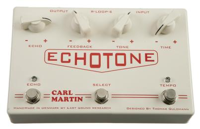
Like the TremO'vibe this is a mains powered unit with a built-in regulated supply. Echo controls the balance between dry and effected signals, Feedback sets the number of repeats, Tone rolls off the treble of the delay line and Time offers manual control of the delay time. The Echo footswitch provides non-true bypass and Select toggles between manual and tap tempo modes.
