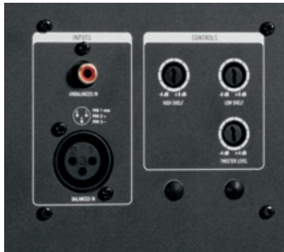
The rear panel plays host to the balanced and unbalanced input sockets, as well as high and low shelving controls and a tweeter level knob.
