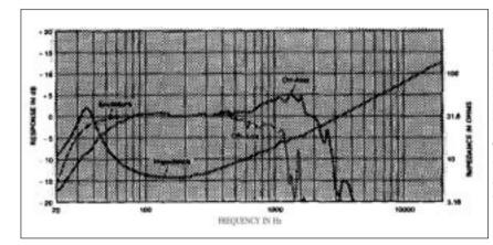
Frequency response contour of the 2241H taken in a hemispherical free-field environment, a closed box of 280 l (10 ft3) internal volume enclosing the rear of the driver. Measured response of a typical production unit, including all peaks and dips, does not deviate more than 2 dB from the above curve. The dotted line represents measured 45 degree off-axis response.
