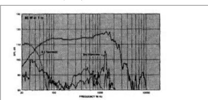
Distortion levels raised 20 dB, measured at 60 watts, 1 meter.
