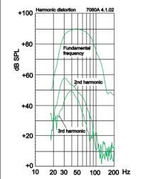
**Figure 4**: 7060A harmonic distortion analysis in free field. In half space the SPL will be 6 dB higher.
