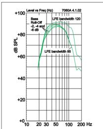
**Figure 3**: 7060A free field frequency response for different bass roll-off and LFE bandwidth settings.
