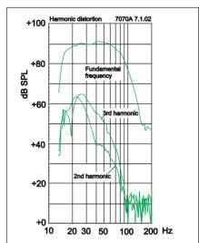
**Figure 2**: 7070A/7071A harmonic distortion analysis in free field. In half space the SPL will be 6 dB higher.
