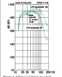
**Figure 1**: 7070A (and 7071A) free field frequency response for different bass roll-off and LFE bandwidth settings.
