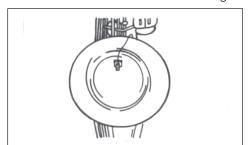
A more mellow sound is achieved by placing and ISOMAX 2 Omni microphone 2-3 inches down inside the bell using double-sided tape. Experiment with the face side down or up (do not cover the screen).
