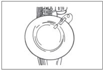
The ISOMAX 2 standard clip also works well when mounted at the top of the bell with the microphone positioned down, pointing inward.
