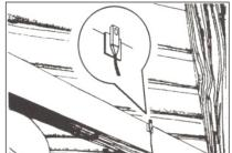
If the lid must be closed or removed, place an ISOMAX 2 Omni on one of the support braces near the middle of the instrument, as shown. Experiment with placement to avoid resonances. For stereo try one on the long support near the middle and one near the upper treble section.
