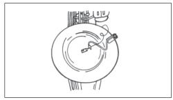
The Countryman Sax clip has foamcovered jaws that tightly grip the bell, with a stiff but adjustable wire that can be positioned at the center of the bell or twisted at the screw to capture sound through the keys.
