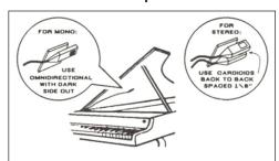
For mono: use double-sided foam tape to attach an ISOMAX 2 Omni facing the lid of the grand piano near the center board, or positioned over the strings on a mic stand. For stereo: place two ISOMAX 2 Cardioid mics on edge 1/8" apart facing left and right. The lid should always be open 3" to 6" (Closing the lid creates a "boxy" sound.)
