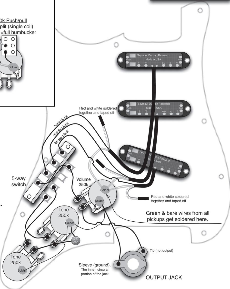
If two pickups sound thin and nasal when used together, chances are, they're out of phase with each other. If you're combining your Seymour Duncan pickup(s) with Fender® pickup(s) in the same guitar, you'll need to reverse the black and green wires on the Seymour Duncan. In other words, solder the black wire to ground and the green wire to the selector switch.
