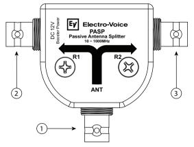
1. BNC jack labeled #1 is where the incoming antenna signal is connected. The cable connected here should be either a CXUF (as part of either RMK1 or RMK2 rack kits), or another
