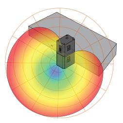
Creating a cardioid subwoofer array forms a more direct radiation pattern and the AIR15s simplifies this with an onboard DSP preset: Just stack two AIR15s subwoofers, with the top subwoofer facing away from the audience and toward the stage, and then set the top subwoofer to use its Cardioid DSP preset. Your two AIR-series subwoofers will then radiate in a directional cardioid pattern, allowing greater steering control over low-frequency energy.
