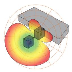
Alternatively, you may prefer to create an end-fire array for even more off-axis rejection. Simply place two AIR15s subwoofers one in front of the other facing the direction to which you want to steer your sub energy and enable the Endfire preset on the rear AIR15s. Need to make a larger subwoofer array? AIR subwoofers are equipped with a variable delay and polarity invert so you can easily build more complex systems.
