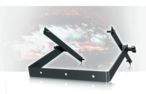
The NuQ122-FY is a matt black, powder coated flying yoke specifically designed to hang the NuQ122 in standalone applications, such as ceiling mounting in bars or clubs, or as an under-balcony fill. The NuQ122-FY consists of: a fly yoke; a pair of side plates, which attach to the sides of the loudspeaker; and a pair of plastic handle screws that secure the fly yoke to the side
