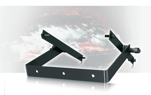
The NuQ102-FY is a matt black, powder coated flying yoke specifically designed to hang the NuQ102 in standalone applications, such as ceiling mounting in bars or clubs, or as an under-balcony fill. The NuQ102-FY consists of: a fly yoke; a pair of side plates, which attach to the sides of the loudspeaker; and a pair of plastic handle screws that secure the fly yoke to the side
