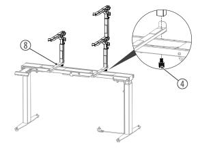
Attach the extensions to the crossbars (8) of the Multi Electric Stand (item no. 491963, separately available) with one 3/8" cylinder head screw (4) each using the Allen key.
