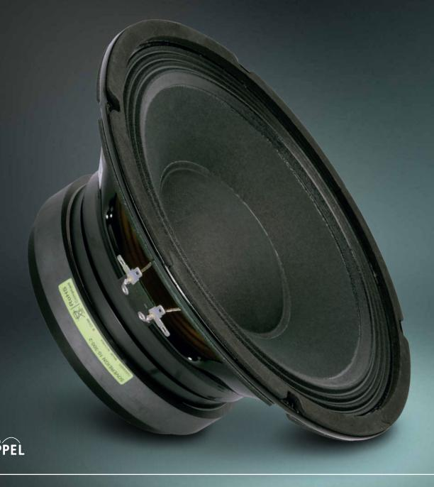
The Fane Sovereign 10-300/2 is a versatile, high power 10 inch loudspeaker for pro-sound mid/bass and bass guitar applications. Working well for mid-range in a small sealed box or as a mid/bass driver in small vented boxes such as the classic bass driver plus horn tweeter. Exhibiting a smooth frequency response, from 45 Hz to 5 kHz, the Sovereign 10-300/2 gives a balanced tonal character when properly matched to appropriate high-frequency drivers.
