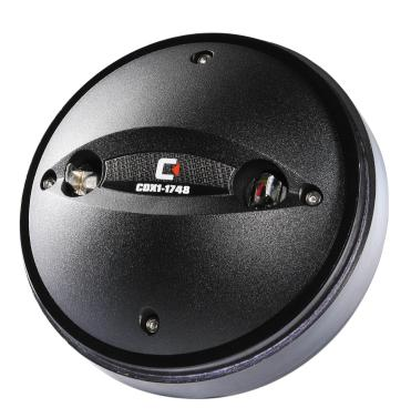
1,600Hz recommended min. crossover freq (12dB/oct) Single piece polyimide diaphragm and surround Sound Castle soft clamping diaphragm assembly Screw fitting
