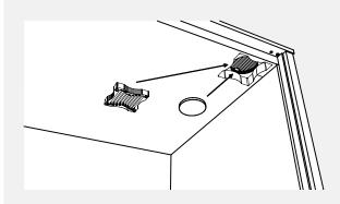
Insert the foam filter in the opening of the isolation booth and attach the ventilation cover with four screws.
