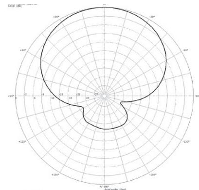
Polardiagramm @ 1 kHz
