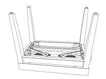
Tighten the nuts manually. Put the bench in a stable position on the floor. Tighten the nuts only then using the included wrench. This ensures that the bench does not shake.
