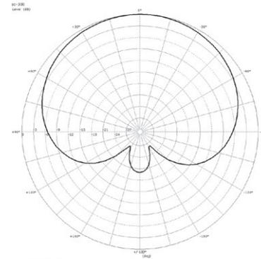
Polardiagramm @ 1 kHz
