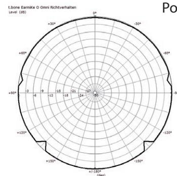
Polardiagramm @ 1 kHz
