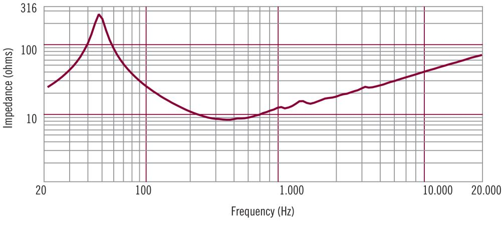
Impedance magnitude curve measured in free air.
